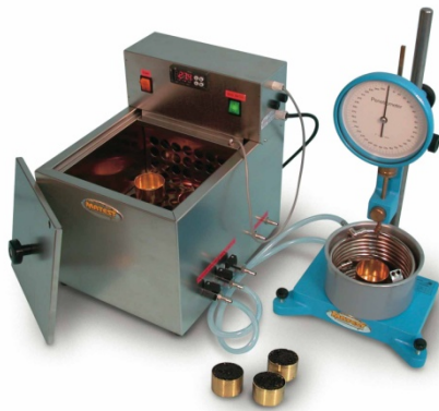
Penetration for Asphalt
