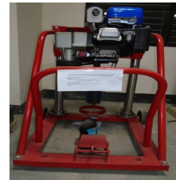
Core Cutting Machine (Petrol Engine Driven)
